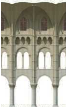
a Laon height of nave, 80'; width of nave, 37'6"; ratio, 2.13:1
